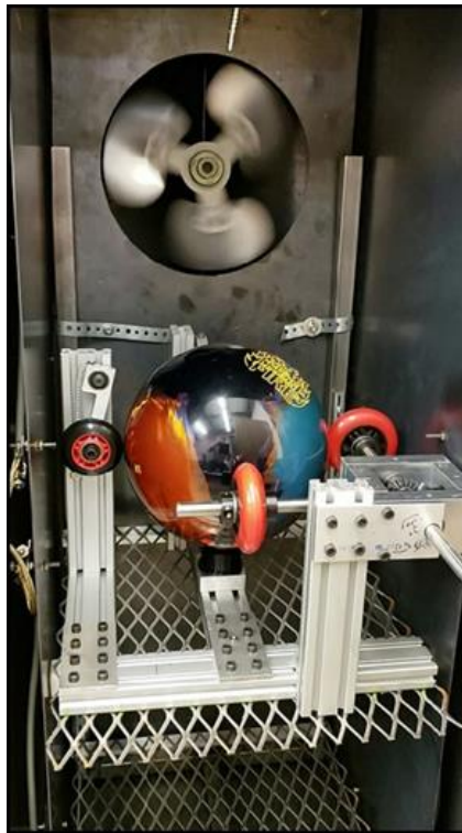
Figure 6: Oven with Circulating air and Ball rotation apparatus
