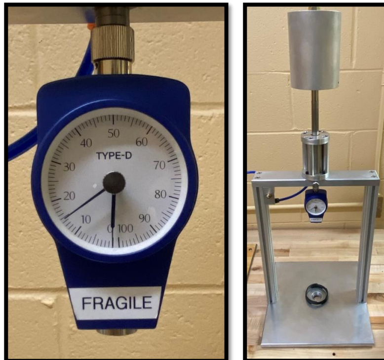
Figure 2: Durometer and the Pneumatic Test Stand
